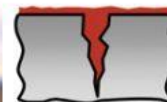
3 Application of penetrant
